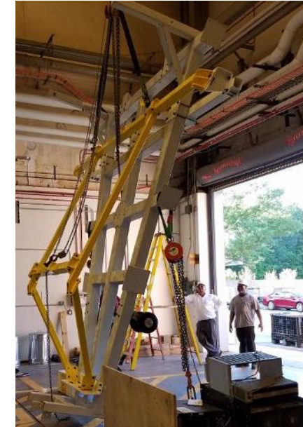
Top Left: DSG installing RICH's electronic panel. Top Right: DSG performing load test of lifting structure (yellow structure). Bottom Left: DSG and INFN collaborators in front of assembled RICH.
