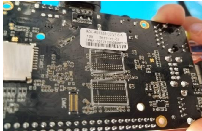
ROC-RK3328-CC SBC card implemented in Hall C control systems
