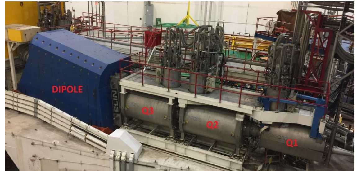
View of the HMS magnets in Hall C
